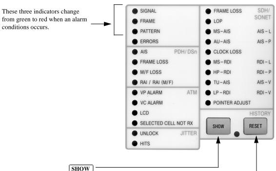
Press and hold this key to view the alarm history. When this key is released the status indicators return to displaying the current status.
