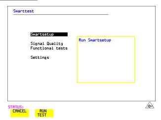
3 With Smartsetup highlighted, press **RUN TEST** to auto-discover information about the receive signal. Or press **CANCEL** to exit Smart Tests.
