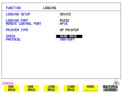
Alternatively, you can use the instrument's pop-up menu feature to make your selection. With the cursor on the required setting field, press **SET** to display a pop-up menu containing the associated values. Use the up or down cursor control keys to make your selection, then press **SET**.
